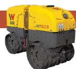
**Double Drum 3,500 lb Remote Control Trench Rollers**
